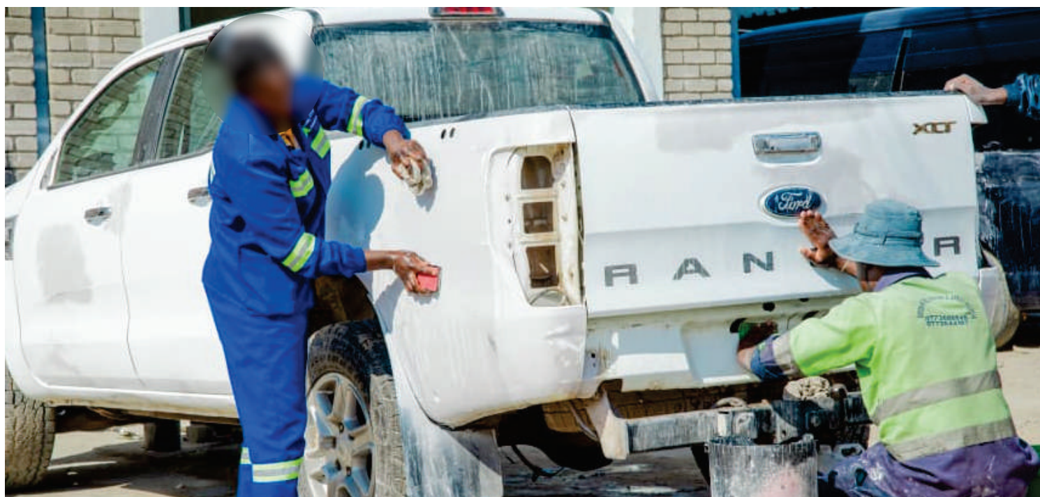
Melinda (pseudonym) doing a panel wipe on a client's car, a key step in panel beating.
